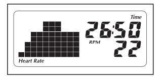
During both programs, the console will regularly compare your heart rate to the target heart rate setting for the current segment of the program. If your heart rate is too far below or above the target heart rate setting, the resistance of the pedals will automatically increase or decrease to bring your heart rate closer to the target heart rate setting. Each time the resistance changes, the resistance level will appear in the display for a few seconds to alert you.
